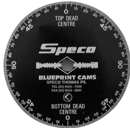
The eight inch diameter degree wheel is designed to insure maximum accuracy in camshaft installations.
